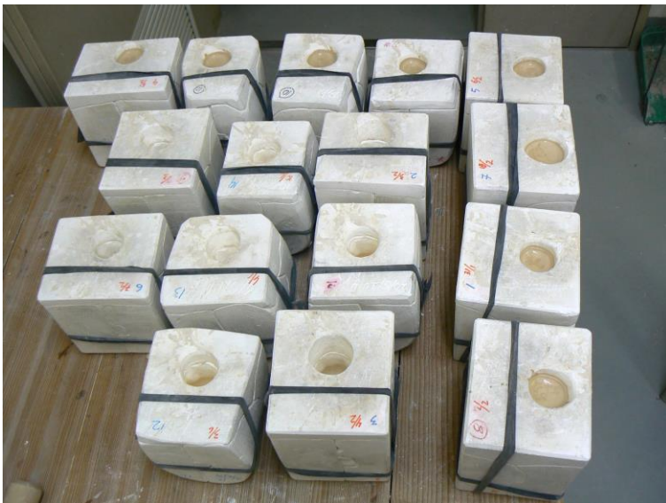
Fig. 4.6 Slip cast molds for the Selves work (page 63)
