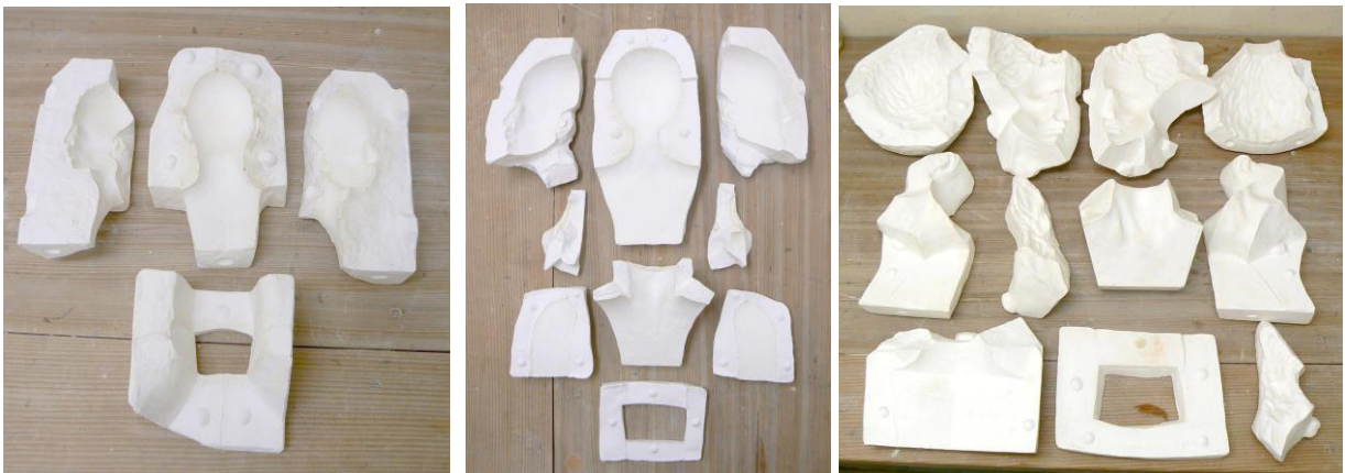
Fig. 4.5 Slip cast molds for head form in three different sizes. (page 63)
