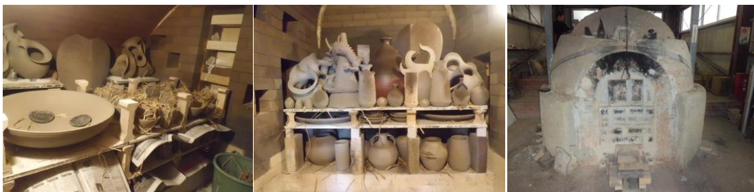
Fig 4.7. Process of loading kiln (窯詰め).
